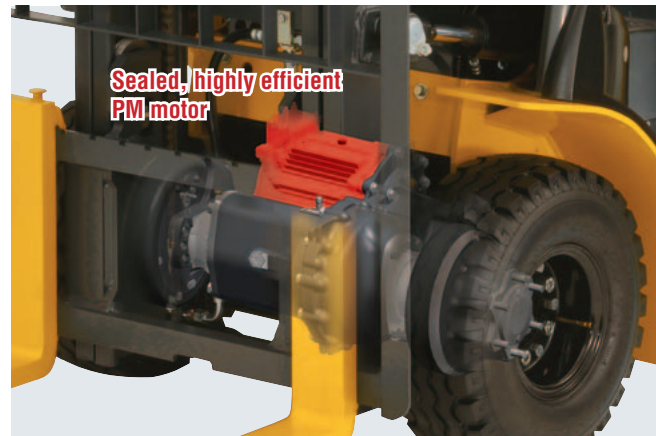
Sealed, highly efficient PM motor
